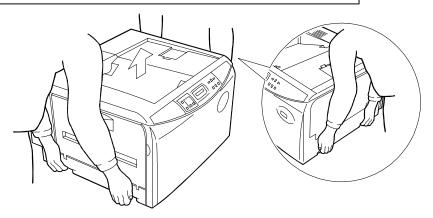
Be sure to lift the printer gently, keeping it horizontal, to prevent toner from soiling the inside of the printer.
